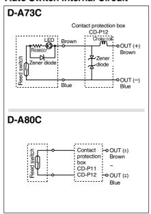
Note 1) Operating load is an induction load. Note 2) Wiring to the load is 5 m or longer. Use the contact protection box in any of the above listed situations. The contact point life may decrease. (Refer to page 1273 for contact protection box.)
