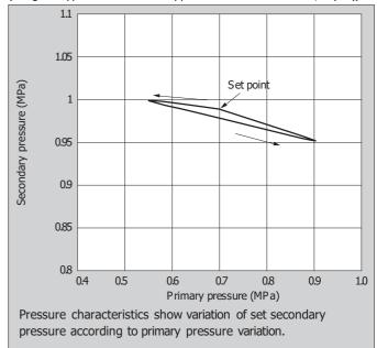
Note: Air booster needs approx. twice secondary side flow rate (max.) for primary side due to structure. Confirm that the instantaneous flow rate is within the curve.
