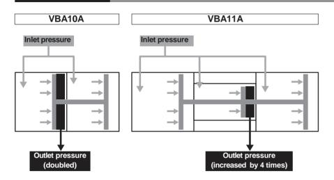
The VBA 1 0 A has two pistons and four chambers.
