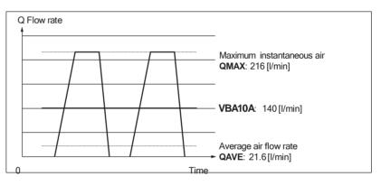
Booster regulator selection and air tank necessity confirmation results
