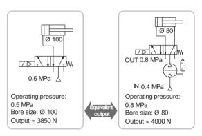
Wh en only one side of the cylinder is used for work, booster regulators can be installed only on the lines that require them to reduce the overall air consumption volume.
